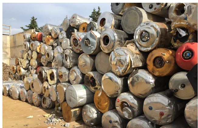
Figure 4: Boilers for manual PU foam removal and processing in refrigerator recycling plants (picture used with the kind permission of the RAL Quality Assurance Association for the Demanufacture of Refrigeration Equipment, 2020).
