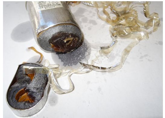
As the dismantling shows, the microwave capacitor is heavily impregnated
