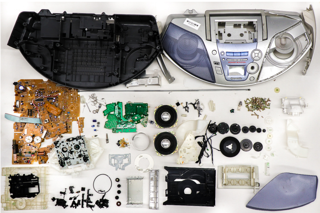
Figure 1: Finely disassembled ghetto blaster
