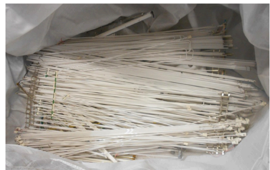
Background lighting containing mercury
