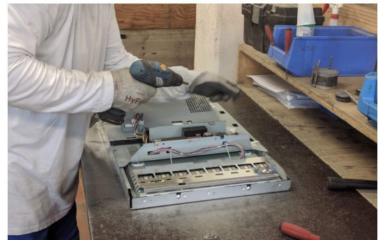
Manually dismantling a PC monitor
