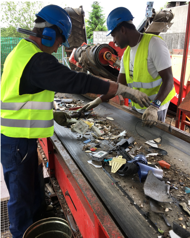
Manual sorting of recyclable and polluting materials from the conveyor belt, after shredding household appliances, at Metabader SA.
