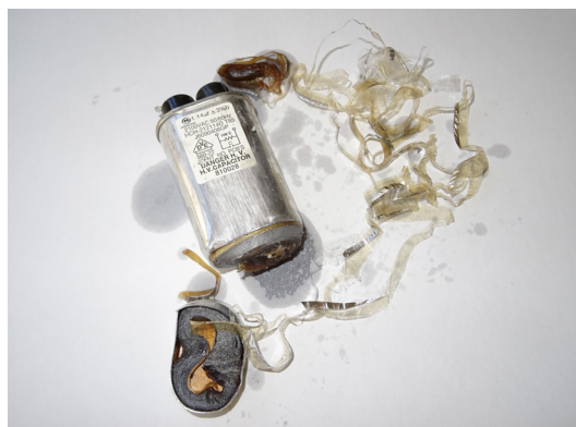
Inner workings of a microwave capacitor
